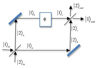
The 50-50 beam splitters are thin black lines and the mirrors are thick blue lines. We assume here that the optical path lengths of the two arms of the interferometer are equal up to a phase-shift  $\phi$  in the upper arm. A single photon sent to the interferometer can be in one of two modes. The quantum system is thus described in a two-dimensional Hilbert space, isomorphic to a spin-1/2 particle.
